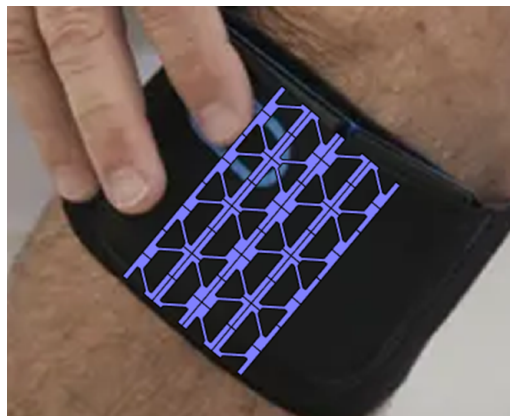
Figure 8. Bistable mechanism to adjust fit of wearable.
