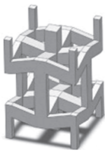
Figure 2: 3D auxetic unit cell.
