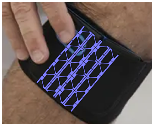
Figure 8. Bistable mechanism to adjust fit of wearable.
