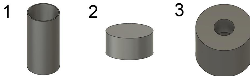
Figure 3. Three samples testing various features. 1: Thin-walled structure. 2: Solid structure. 3: Solid and thick-walled structure
