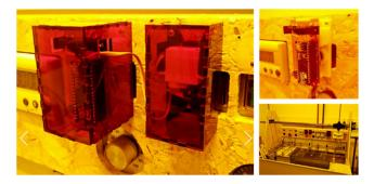
Figure 1. Left: a pushbutton on the left and a rocker switch on the right automated with modules. Up right: a button pusher module uncovered. Down right: A printed circuit board through hole plating machine automated with the modules. The entire automation system can be removed from the machine in one piece
