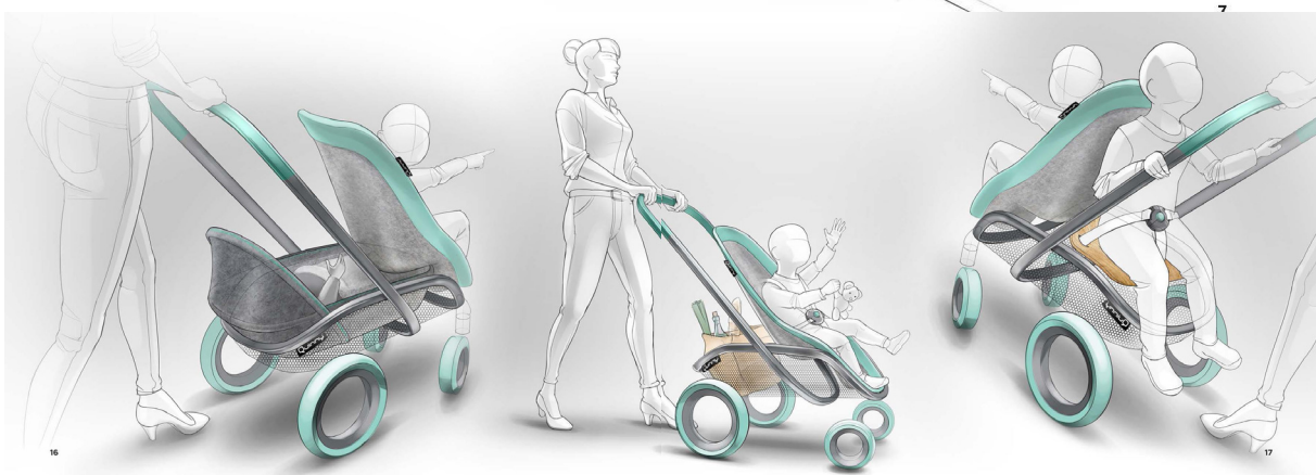
Figure 9. Preliminary positions of two children. Not so much exploratory in the product, as exploratory in use and package configuration; the ways in which two children, or one child plus luggage, can be positioned in a stroller.
