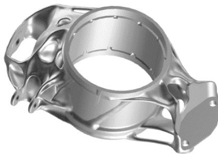
Figure 3. Wheel carrier of student's race car
