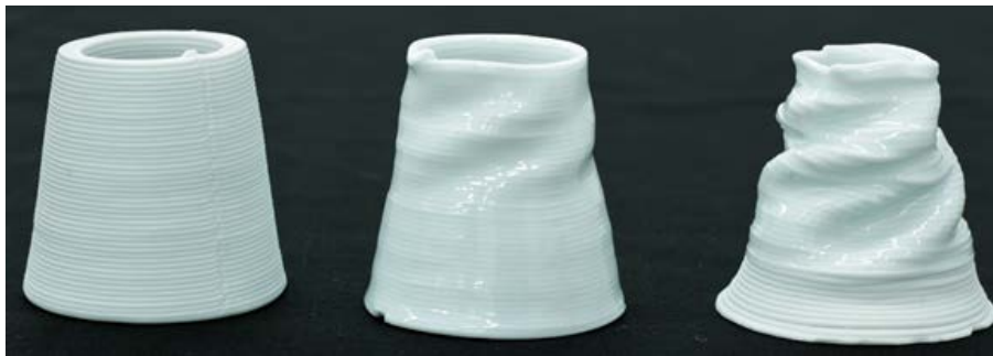
Figure 8 – Experiments with extrusion of ceramic materials (courtesy of ADDlab).
