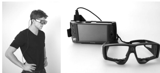
Figure 1. Mobile eye tracking glasses and recording unit (SMI, 30Hz)
