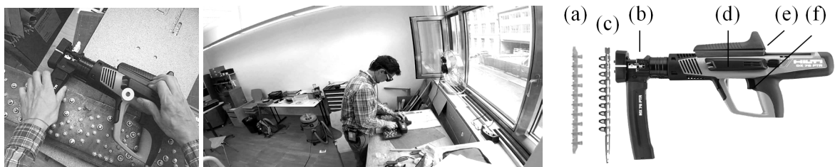
Figure 4. Eye tracking perspective; third-person perspective; fastening tool with fastening strip(a), magazine(b), cartridge strip(c), cartridge guideway(d), cycling grip(e) and trigger(f)
