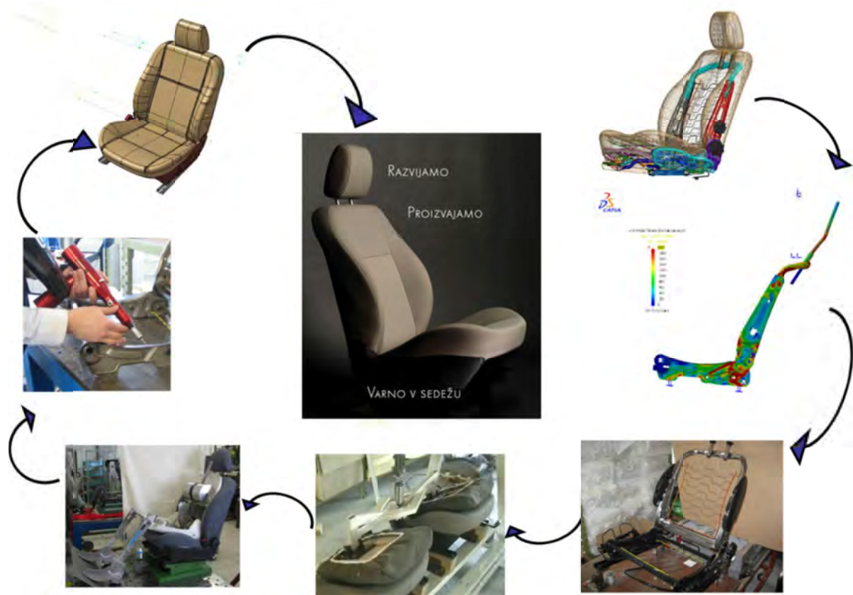
Figure 3. Design and development stages according to the system of concurrent engineering
