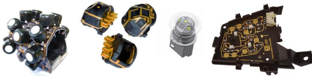
Figure 4. Motor cycle switch (left, Kromberg & Schubert) solar sensor (middle, Harting), steering-wheel switch (right, TRW) [Franke et al. 2011]
