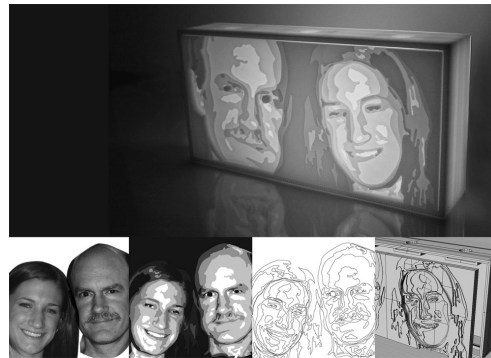
Figure 4. The process of translating a digital image into a physical relief display
