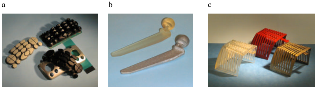
Fig. 4. Example parts manufactured in Rapid Tooling technologies: a – flexible keyboard cast in polyurethane with properties equivalent to elastomer, b – resin and aluminum prototypes of a medical implant, c – resin prototype, wax copy and a framework cast in brass
