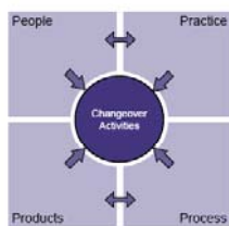
Figure 2. The 4Ps of changeover: Main influences on changeover capabilities of manufacturing equipment
