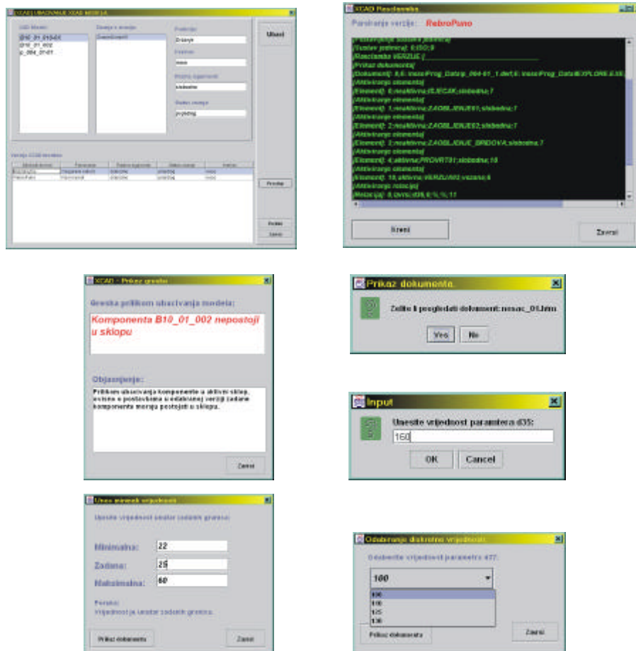
Figure 11. Screenshots of the system windows during the insertion of the XCAD part (upper two pictures) and the dialog boxes for the control of the parts parameters (lower five pictures)
