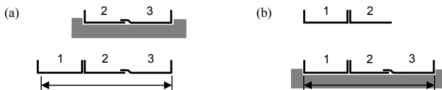
Figure 1. Two assembly sequences for a car floor pan design [1] where total length is critical. In (b), the total length is controllable while it is not in (a).
