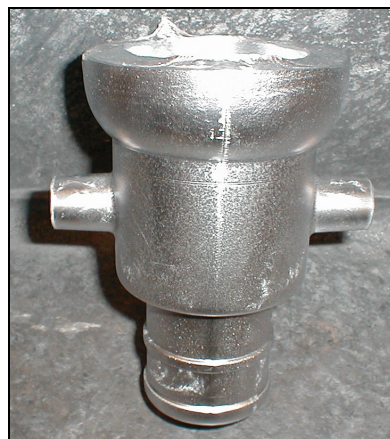
Figure 8 A casting of the presented case study from Al-Si7Mg, Source: Walter Frank & Sons Ltd., Barnsley, UK
