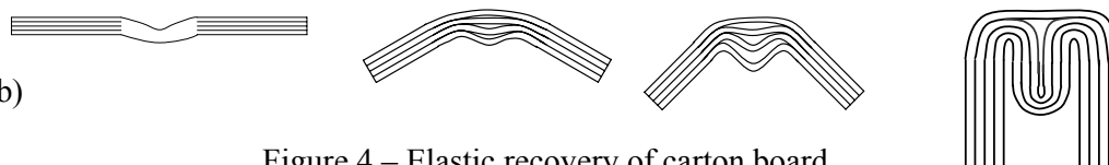
Figure 4 – Elastic recovery of carton board
