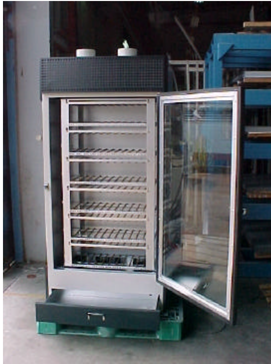
Figure 1. Finished Alpha Prototype of the Burn-in System (Chamber with PCB Cage inside)
