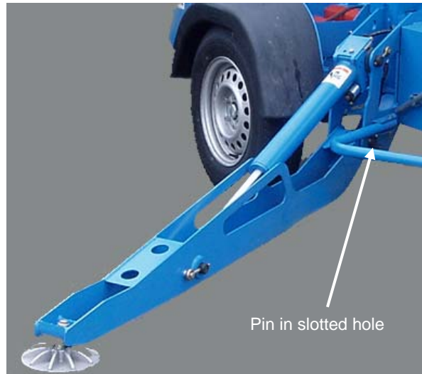
Figure 8. 4B1 (4 th Generation Stabilisers, Company B – Type 1 - Hydraulic, sliding pin sensing)
