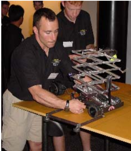
Figure 1. Different concepts at the 2002 National Final in Sydney's Powerhouse Museum in 2002. The task was to traverse 3.0 m, then drop a tennis ball down the 1.0 m high vertical plastic pipe in the minimum possible time. (a) The top photograph shows the winning device, which used pneumatically-powered telescopic tubes and dropped the ball to the bottom of the pipe in 1.0 sec. (b) This device used guide wheels running on the edge of the track to ensure lateral accuracy. It dropped the ball as it ran past the pipe. (c) This design employed a large V 'catcher' to guide it into position on the pipe. Unfortunately it failed to rise to its design height, did not align correctly, and the ball can be seen falling outside the pipe.
